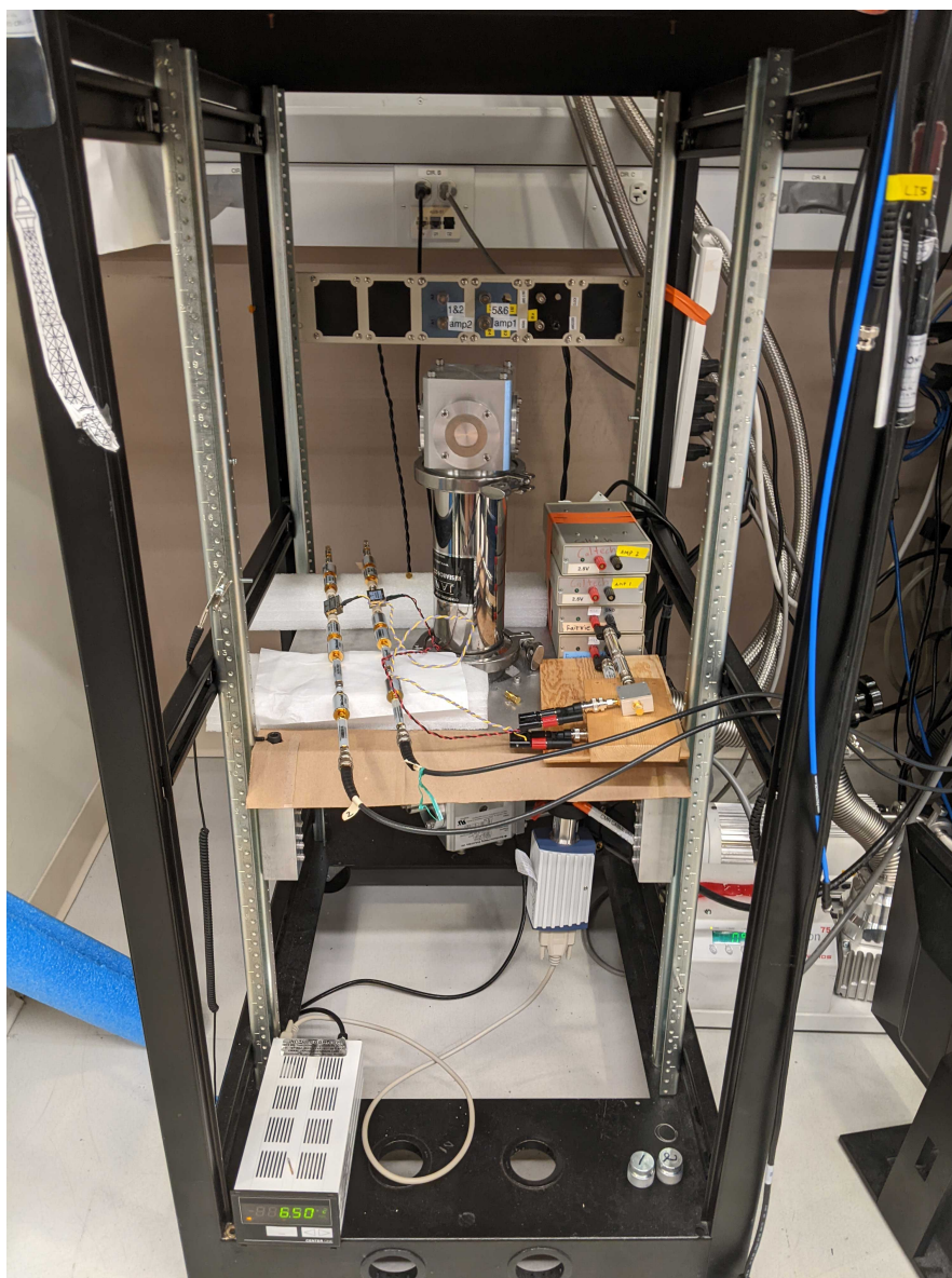
Figure H.1: Image of the Sumitomo cryostat mounted in its rack, with the vacuum can installed.
