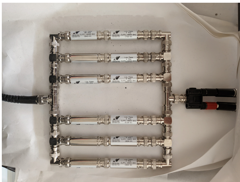
Figure 4.4: A filter bank of 6 series-pairs of Crystek low-pass RF filters used for filtering out RF noise for high-current heater lines for the cryostat. The 6 rows of filters are necessary to split the heating from the large DC current to avoid burning out the filters.
