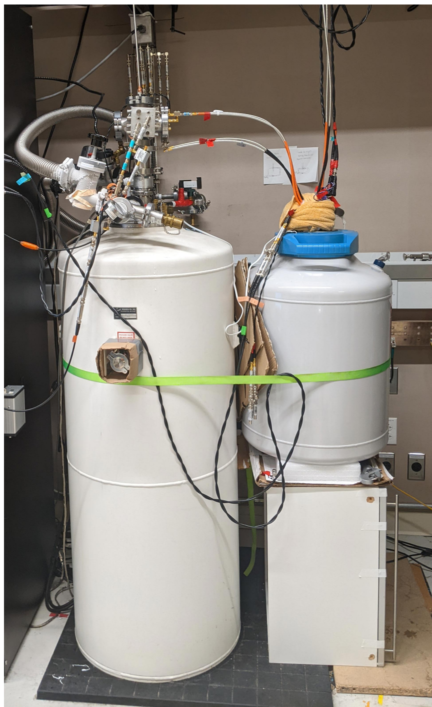
Figure H.4: Images of the Janis setup, with the main cryostat on the left, and the liquid nitrogen dewar with LNA electronics on the right.
