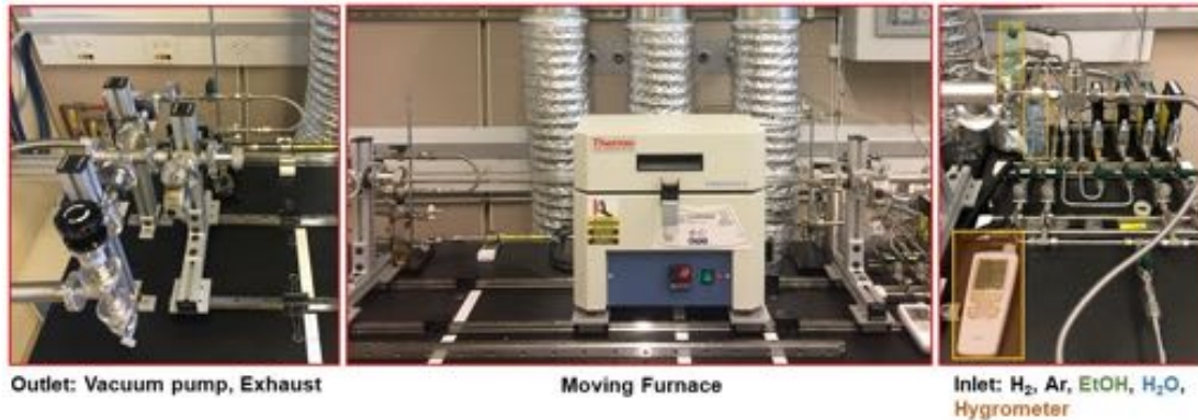
Figure 3.2: The carbon nanotube growth furnace. The furnace is composed of three sections highlighted in red. Left: outlet for vacuum pumping to evacuate the tube furnace and for growth gas exhaust. Middle: moving furnace for fast heating and cooling. Right: inlet that includes four mass/gas flow meters for hydrogen and argon, two bubblers for ethanol and distilled water, and a hygrometer.
