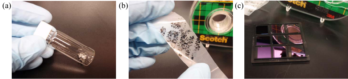
Figure 2.3: (a) Bulk kish graphite used for graphene exfoliation. (b) A piece of tape prepared with graphite and ready for pressing onto a chip. (c) Clean Si/SiO 2 substrates for graphene exfoliation.
