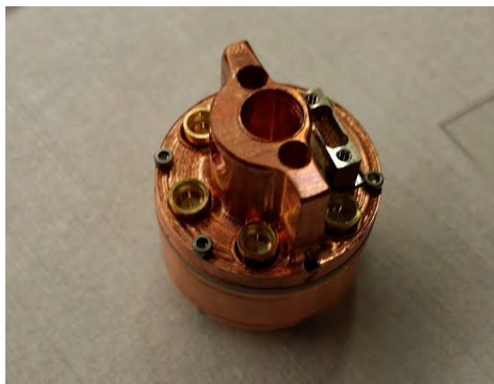
Figure A.4: Sample package mounted to the custom adapter made for the Oxford cryostat. Adapter has two machined holes to house a heater and thermometer. Entire package is then affixed to the end of a long SS thin-walled tube and lowered into the Oxford VTI.
