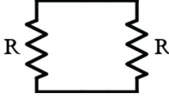
Figure 2.1: Schematic of Nyquist's famous thought experiment. Two resistors in thermal equilibrium are connected end to end and allowed to transfer energy between them via thermal current fluctuations.
