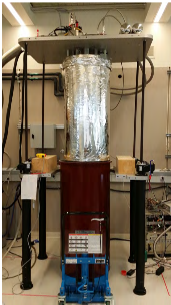
Figure A.8: Image of the Leiden cryostat being disassembled. The four electrically controlled legs are extended, lifting the entire system for easy maintenance.
