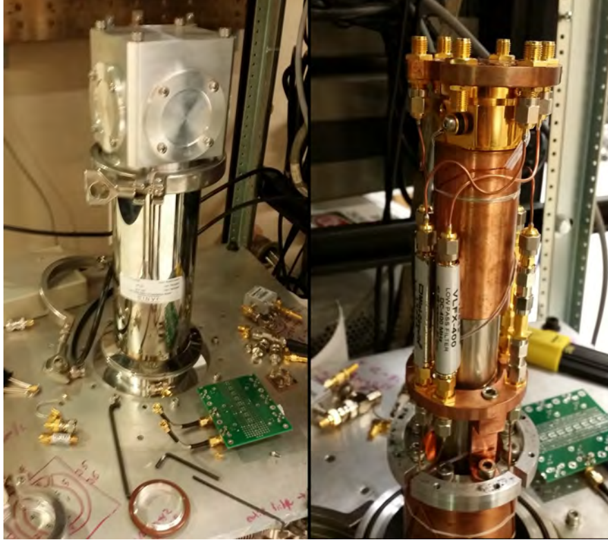
Figure A.3: Janis SHI-4 cryocooler used in parts of this dissertation. (Left) image of the closed system sealed and under vacuum. Optical windows are available but are blocked for these experiments. (Right) image of the opened system exposing the RF semi-rigid coax cables. The sample package is mounted onto the top plate which is cooled via a closed cycle ^4\text{He} system and the temperature is set using a heater, thermometer, and Lakeshore PID controller. Low-pass filters are placed at the mid temperature plate to reflect room temperature noise.
