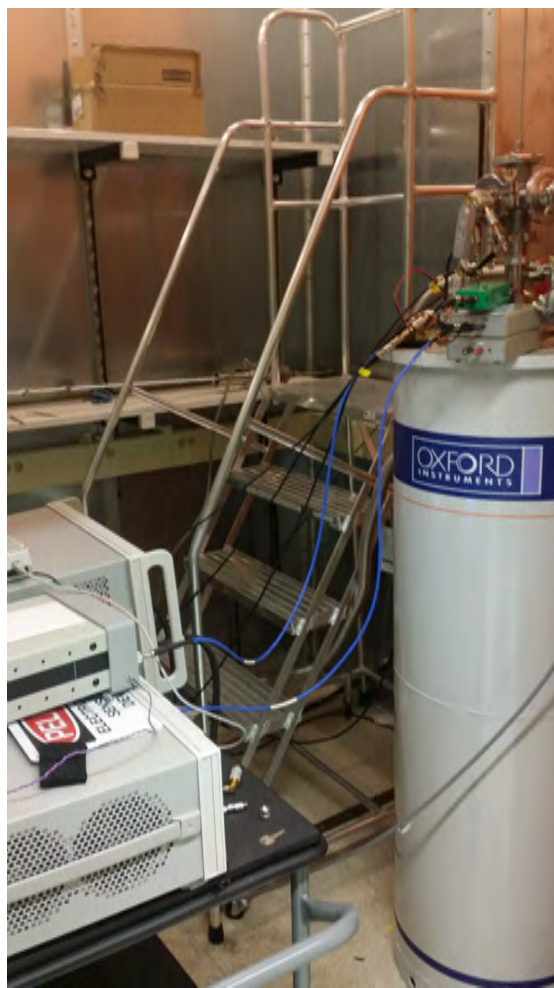
Figure A.6: Image of the Oxford cryostat with VTI and RF probe during a measurement. All electronics are kept at room temperature. The entire fridge is housed inside a shielded metal room.
