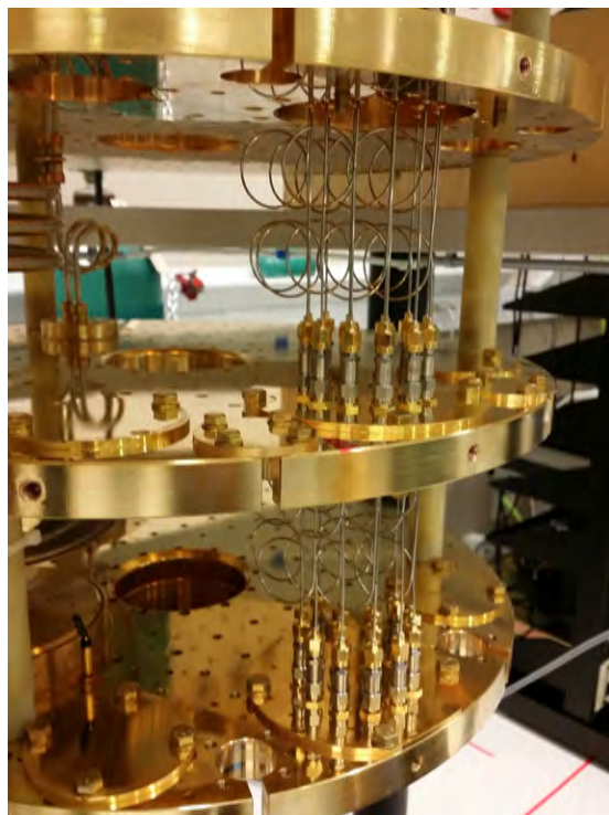
Figure A.11: Image of the microwave lines inside in the body of the Leiden cryostat. Shown here are the 14 excitation lines connecting the still plate to the mixing chamber plate attenuated at every stage. Not shown are the 2 superconducting measurement lines installed alongside these without attenuators.
